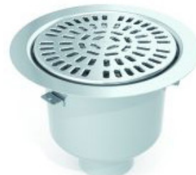
Heavy 110 R Prod. code: 7102837 Diameter: 220mm Outlet: Vertical 110mm
