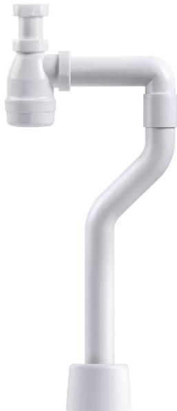
S-Bend water trap kit designed for floor connection with a 1¼" bottle trap and a 40mm diameter outlet pipe. This water trap kit allows for floor installation directly below the vertical waste, and 320mm to the side. Comes with floor cover.
