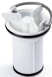
Plastic NOOD water trap for Safe Overflow. The water trap is a mechanical odour stop designed to close when there is no water flow, thus preventing odours from escaping through the drain, even when dried out. It is therefore suitable for environments which have little or no water supply for longer periods of time. When water is flowing through, the water trap opens automatically. It can be removed from the outlet gully for easy cleaning and maintenance.
