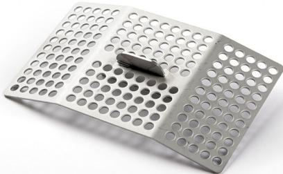
Filter basket in acid resistant stainless steel with a volume of 0.33 liters. The Filter basket is used to collect particles larger than 5 mm, e.g. leaves, so they do not fill up the water trap. The Filter basket is picked up for emptying and reassembled.
