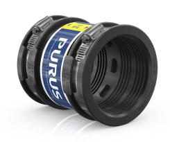
Standard couplings are used to connect two waste water pipes with the same dimension, as well as waste water pipes with the same or different materials and surface structure. Standard couplings are suitable for vertical and horizontal installation. They have two sides, both with hose clamps for external installation of waste water pipes. They are easy to install in a few minutes and are approved for concealed placement. The material is UV-resistant.
