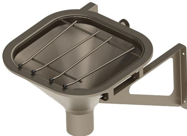
V151 Slop sink is manufactured in stainless steel and is for wall installation. It comes with grates and brackets as well a rinsing device for cleaning. The V151 Slop sink is designed for use in cleaning rooms, as well as in cleaning areas in hospitals, campsites and public toilets.
