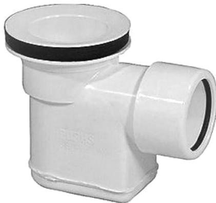
Shower/bath trap with strainer valve. It has a 1½" connection and is designed for 40mm diameter outlet pipes.
