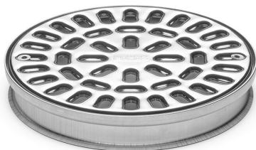
The Resin Ring 150 is made of acid-resistant stainless steel. It is for resin, micro-cement and micro-concrete floor finishes and is suitable for all Purus floor drains with a 150mm grate diameter. Comes with a lockable grate and locking accessories. Raises the floor drain by 3mm.
