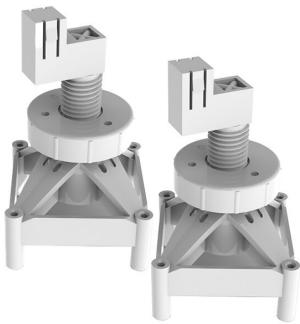
The Purus support (2 pieces) is designed for installing Purus' side outlet plastic floor drains in concrete floors. The support can be adjusted in height to approximately 60mm, with an extra extension piece to extend to approximately 110mm. The Purus support is attached to the drain with a nail or screw, and can then be height adjusted using the nut.
