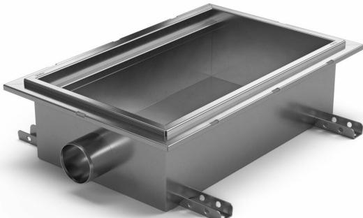
Purus channel combo is made of acid-resistant stainless steel with side outlet Ø75 mm for installation in concrete. The floor channel is 300x300x150 och är avsedd för klinkergolv som ytskick. There is always residual water in the channel about 50 mm of water forms the water trap in the bottom of the channel and is equipped with a cleaning plug. The floor channel requires an almost continuous flow to function properly. Unsuitable in environments that set hygiene requirements.
