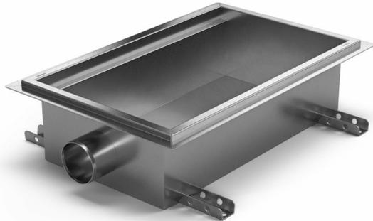
Purus channel combo is made of acid-resistant stainless steel with side outlet Ø110 mm for installation in concrete. The floor channel is 300x300x200 och är avsedd för massagolv som ytskick. There is always residual water in the channel about 50 mm of water forms the water trap in the bottom of the channel and is equipped with a cleaning plug. The floor channel requires an almost continuous flow to function properly. Unsuitable in environments that set hygiene requirements.
