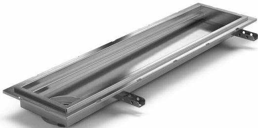
Purus channel 200 is a floor channel made of acid-resistant stainless steel for installation in concrete. The floor channel is 600×200 mm with a deep end outlet and is intended for tile flooring. The floor channel needs to be supplemented with a grating/grid depending on the environment and outlet house in plastic or acid-resistant stainless steel.
