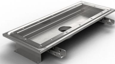
Purus channel 150 is a channel made of acid-resistant stainless steel for installation in concrete floors. The channel has a central outlet and is intended for vinyl floors as a surface layer. Supplement with gully base in plastic or acid-resistant stainless steel and mesh grate for higher load classes or grating for K3 (300 kg) load.
