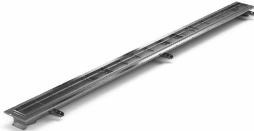
Purus channel 100 is a floor channel made of acid-resistant stainless steel for installation in concrete. The floor channel is 600×100 mm with an end outlet and is intended for tile flooring with glue flange. The floor channel needs to be supplemented with a strainer/grating due to the environment and an outlet house made of plastic or acid-resistant stainless steel.
