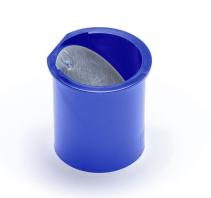
Blue plastic PUM membrane insert for vertical installation in inlets of 40mm diameter pipes. Spare part for Purus Universal Membrane products. The membrane acts as an odour barrier and is integrated within the waste, where it remains closed until opened by water flow. It is easy to clean, saves space in the installation area and has a high flow rate. Type approved by RISE.
