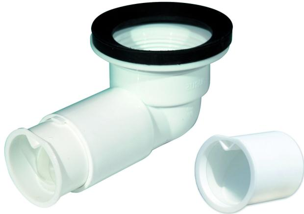
The PUM bath waste bend in plastic has a 1½" connection and is designed for 40mm diameter outlet pipes. It comes with a gasket. The odour barrier (membrane) is integrated in the waste bend and is positioned within the pipe for easy cleaning and maintenance. The waste bend replaces the usual cup-style water trap, saving space in the installation area. It should be installed in conjunction with standard vertical wastes.
