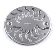
Round stainless steel grate for vinyl flooring with the Wave design. Designed to fit Purus' floor gullies with a 130mm grate diameter. The grate is manufactured to ensure a good flow rate and has a K3 load class. The Wave grate can be locked when used with the appropriate locking nuts.
