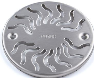
Round stainless steel grate for vinyl flooring with the Wave design. Designed to fit Purus' floor gullies with a 130mm grate diameter. The grate is manufactured to ensure a good flow rate and has a K3 load class. The Wave grate comes with a locking device for securing to the clamping ring.
