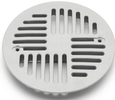
The Art Deco 130 is made of 100% recycled plastic in grey. For Purus floor drains with a 130mm grate diameter. It is suitable for vinyl floor finishes. The grate is designed to withstand a good flow rate and has a K3 load class.
