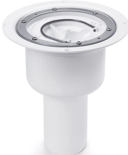
The S-Series Brage is a floor drain with a 75mm vertical outlet for installation in wooden or concrete joists. The S-Series Brage floor drain comes with a removable water trap and stainless steel clamping ring. It also comes with a protective cover that is intended to prevent any concrete or debris from installation from entering the drain.
