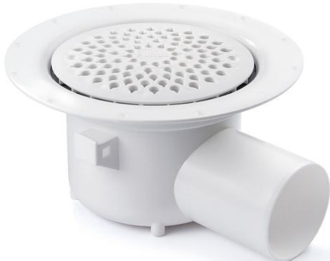
The Oden floor drain has a 75mm sideoutlet and is for installation in wooden or concrete joists. The Oden floor drain comes complete with a removable water trap, clamping ring and plastic grate. It also comes with a protective cover that is intended to prevent any concrete or debris from installation from entering the drain.
