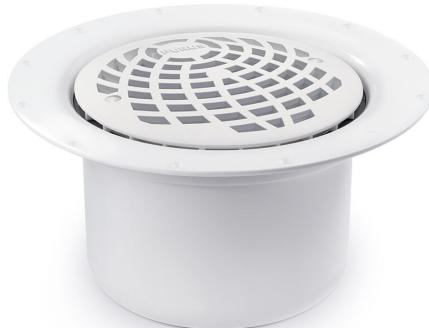
The Duschbrunn 50 Vertical floor drain has a 50mm vertical outlet and a total height of 98mm. It is suitable for installation in wooden or concrete joists. The Duschbrunn floor drain comes complete with a removable water trap, clamping ring and plastic grate. It also comes with a protective cover that is intended to prevent any concrete or debris from installation from entering the drain.
