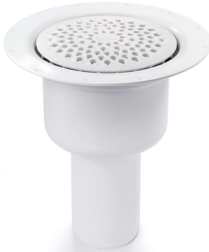
The Brage 75 Vertical floor drain has a 75mm vertical outlet and is for installation in wooden or concrete joists. The Brage floor drain comes complete with a removable water trap, clamping ring and plastic grate. It also comes with a protective cover that is intended to prevent any concrete or debris from installation from entering the drain.
