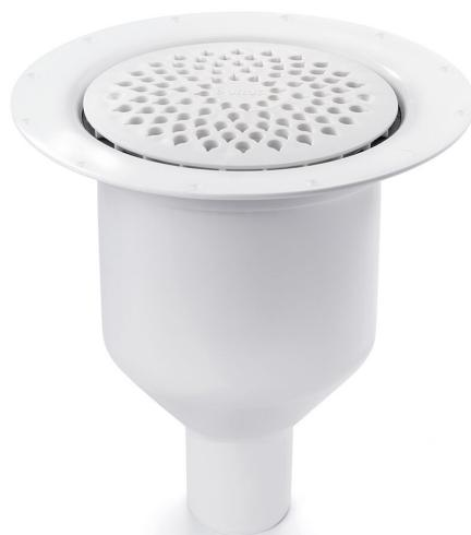
The Brage 50 floor drain has a 50 vertical outlet and is for installation in wooden or concrete joists. The Brage floor drain comes complete with a removable water trap, clamping ring and plastic grate. It also comes with a protective cover that is intended to prevent any concrete or debris from installation from entering the drain.
