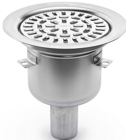
The Balder 50 R floor drain has a 50mm vertical outlet and is for installation in wooden or concrete joists. The Balder floor drain comes with a stainless steel water trap, clamping ring and stainless steel grate. It also comes with a protective cover that is intended to prevent any concrete or debris from installation from entering the drain.
